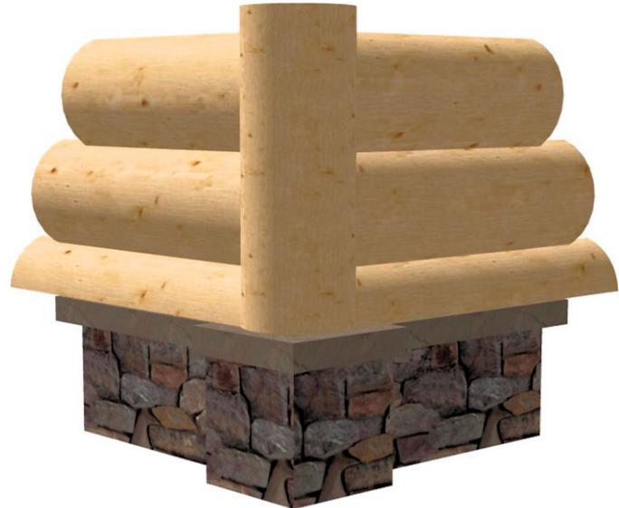
Half-height starter log on built-out stone face base to "support log wall."
