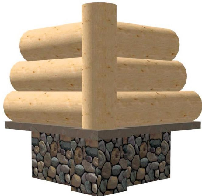
Full-height starter log on built-out stone face base to "support log wall."
